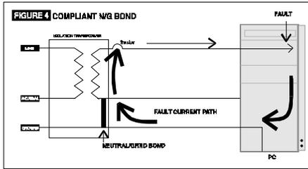
Since the neutral and ground are shorted and the return paths are short, there is not voltage drop created by the operation of normal mode suppression.
