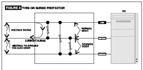
to the impulse that triggered it. In essence, a normal mode event has been converted into a common mode event. This is not a problem with a transformer-based device.
