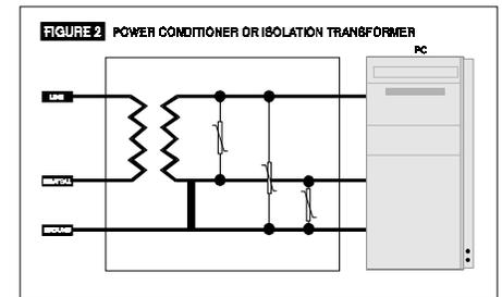
suppressors have been added. This helps knock down large surges that might kill the power supply. Depending on the source of the MOVs, the let through voltage may be as high as 400 to 600 volts before they clamp the energy from line to neutral. This is good enough for normal mode protection, but far too large to protect logic chips.
