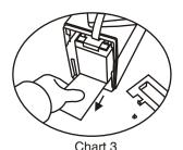
After removing the front cover, follow Chart 2 to remove partition by removing the screw. Then follow Chart 3 to pull out battery by pulling attached white vinyl sheet. Disconnect the wires connected to the battery. Be sure to replace the same type of batteries and dispose of old batteries properly at an appropriate recycling facility.
