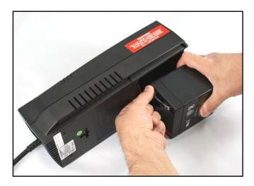
8 Slide the battery back in its place. Slide the cover back in and screw it tightly.
