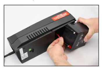
WARNING: Do not make any contact with the battery terminals with the screwdriver or any other metal materials like watches, rings, etc. Electric shock could occur and it could cause harm to you and the battery.
