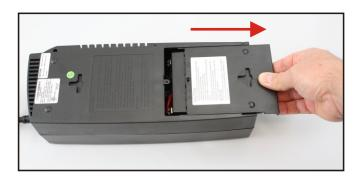
5 After removing the battery cover, tilt the UPS as shown below and gently slide the battery slightly until you have room to disconnect the wires.
