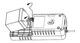
Disconnect the two wires connecting it to the Office Plus UPS and replace it with the same type of batteries. Dispose of the old batteries properly at an appropriate recycling facility.
