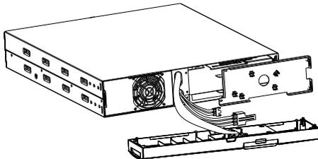
5. Pull the battery pack out onto flat area.
