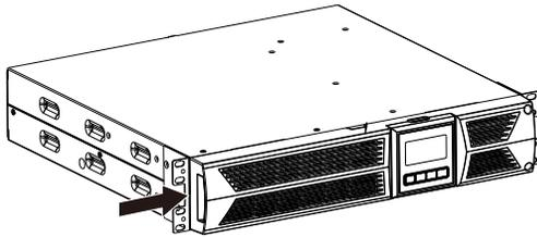
2. Assemble the rack rails with the rack-mounting.
