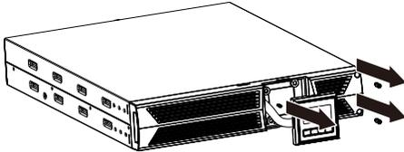
2. Slide and pull the front panel leftward and then take it off.
