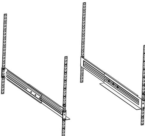
3. Slide in the UPS into the rack rail and lock it in the rack enclosure.
