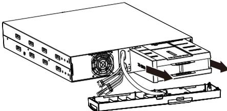
6. Install new battery pack into UPS.
