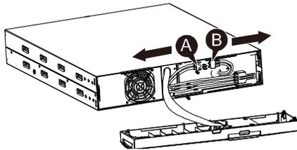
4. Remove the right inner battery bracket.
